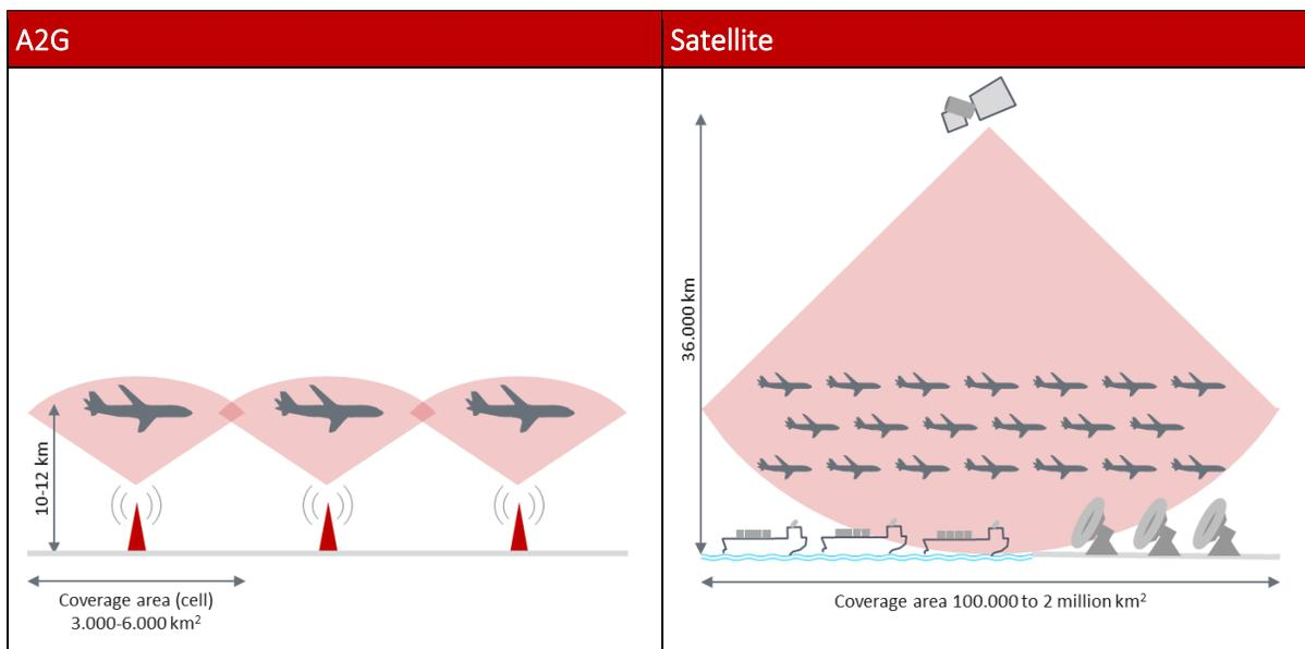
An A2G solution based on 3GPP standards has compelling advantages over satellite systems and inherits the fast feature evolution of standard terrestrial networks and the economies of scale resulting from large scale public mobile network deployments. When comparing both technologies with each other the advantages of A2G communications become obvious:
