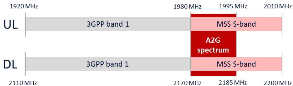
This band, commonly referred to as Band 65a (i.e., the lower half of band 65), allows achieving a downlink throughput of 100 Mbps for each connected aircraft. The required ground network and aircraft terminal equipment is available and in extensive commercial use in Europe. Assigning the same band in other markets will assure:
