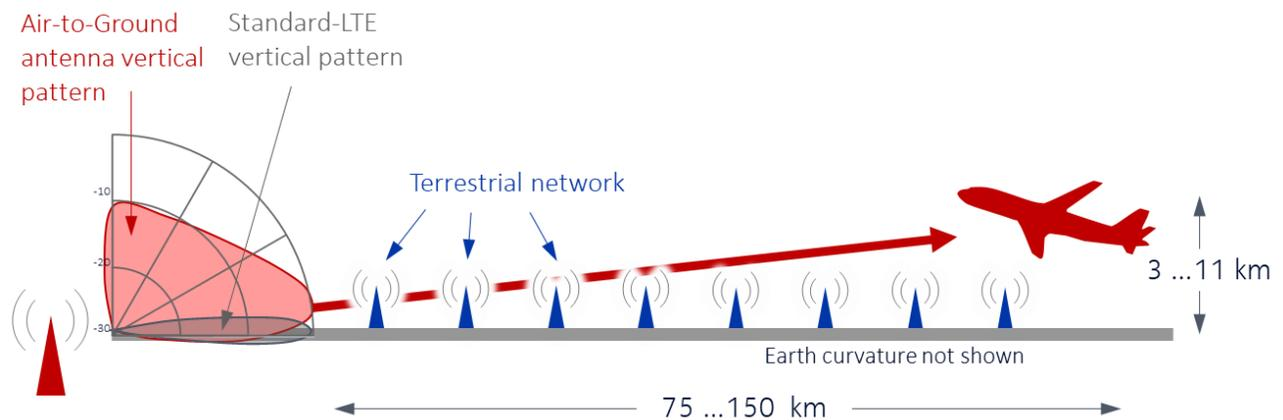
For the European Aviation Network, which is the first A2G network based on 3GPP standards, 2x15MHz of Frequency Division Duplex spectrum in the 2.1GHz range were assigned:
